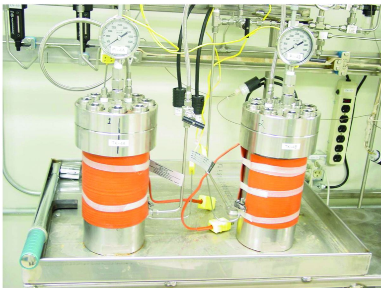
Figure 4. Pilot Plant Extraction Vessels Used for Uranium Recovery from Incinerator Ash
